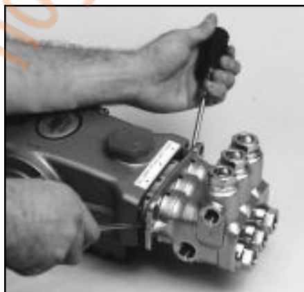
Removal of Manifold Head from Crankcase
